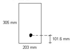
Q.3 (a) Design a simply supported (Type-II) pretensioned prestressed concrete beam for flexure only as per IS:1343-1980 with total moment  $M_T$ =435 kN-m (including an estimated self-weight moment  $M_{sw}$  = 55 kN-m). The prestress at transfer is 1035 N/mm<sup>2</sup> and at service is 860 N/mm<sup>2</sup>.
