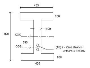
The properties of the sections are as follows  $A = 159,000 \text{ mm}^2$   $I = 1.7808 \times 10^{10} \text{ mm}^4$ .  $Ap = 960 \text{ mm}^2$ .
